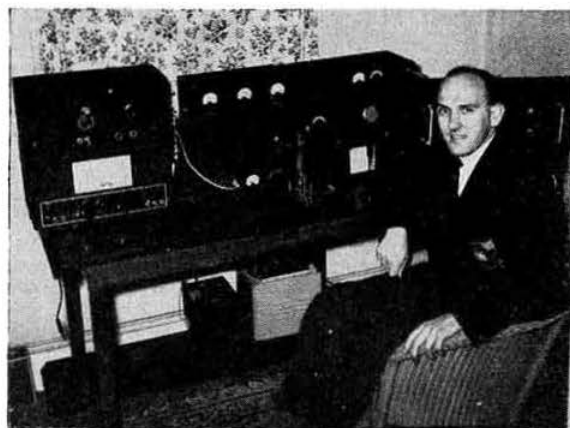
The leading station in the low power section, GW3AHN of Cardiff. In this picture, the Eddystone 5640 receiver is at the left, with the v.f.o., n.b.f.m. and speech clipper standing on top. To the right is the exciter unit using a Labgear multiplier with the a.t.u. above, and the band switched 807 p.a. standing on a TUS type v.f.o. not now in use. The rack on the extreme right contains (from top to bottom) an experimental p.a., speech amplifier and modulator and the p.a. power supply giving 400 volts at 150mA and 500 volts at 200mA.
